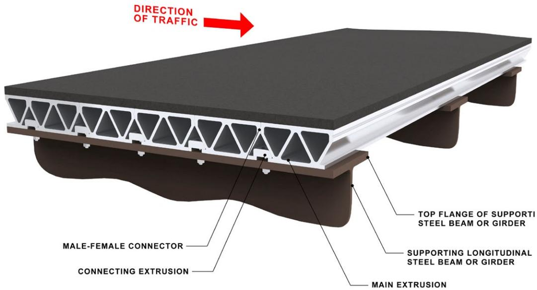
Figure 2. Extruded aluminum bridge deck system.
