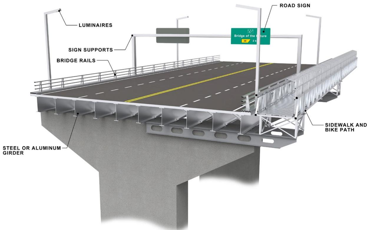
Figure 3. Use of aluminum in secondary bridge components.
